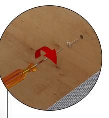
Using the screwdriver connect bases into position using 2x screws (E).
